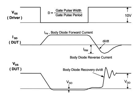
Body Diode Forward Voltage Drop
